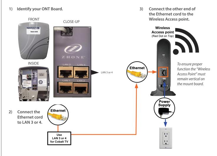
4) Plug the power cord into an outlet. The Power LED light will turn on, indicating the unit is powered. You have completed set up for the Main Access Point.
